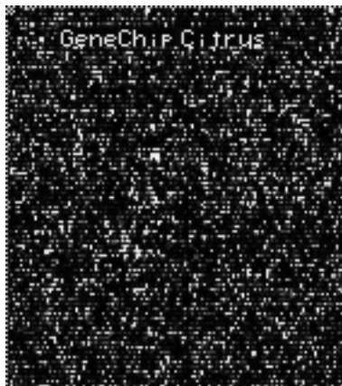
Figure 1. Image of about 2% of a Citrus GeneChip® used for analysis of iron chlorosis tolerance. Each visible dot is a probe (25-base DNA fragment) from a gene that is expressed in roots during iron chlorosis stress. Dark areas are probes from genes that are not detectably expressed under these conditions. This microarray contains an embedded chip identifier “GeneChip Citrus”.
